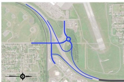
Princess/Neebing - Roundabout ramp terminal on west side of highway
