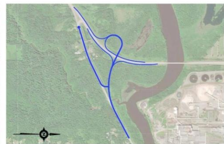
Chippewa Road -Trumpet B interchange 500m north of existing and realign Chippewa road
