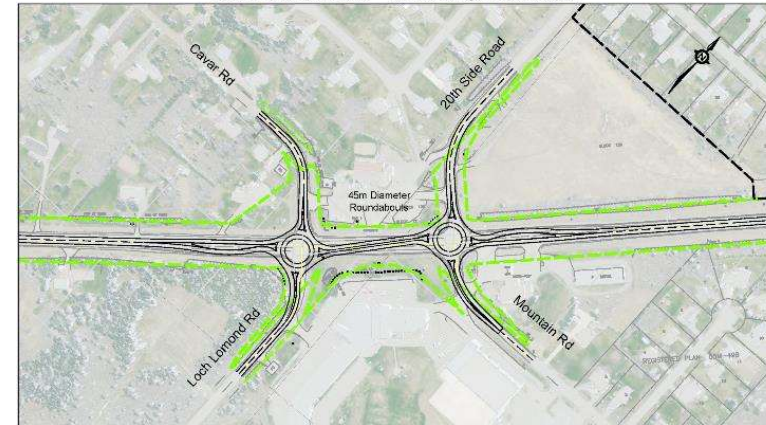
Alternative 1B Dual Roundabouts - At Existing intersection
