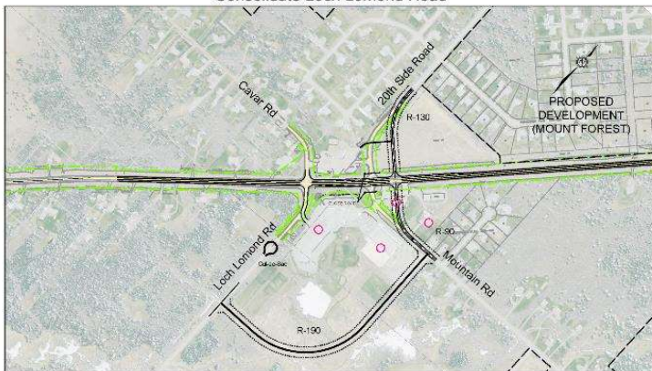
Alternative 3A - Conventional Intersection Relocate Mountain Road/20th Sideroad Intersection and Consolidate Loch Lomond Road
