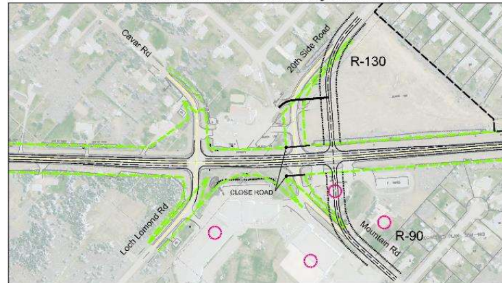
Alternative 2A Conventional Intersection With Realigned Sideroad
